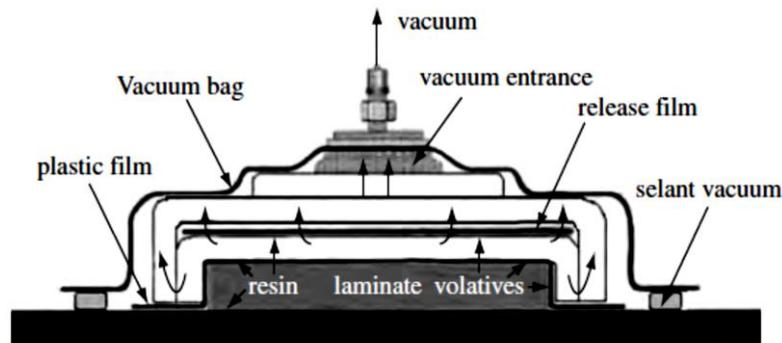
**Fig 3. Schematic Representation of Vacuum bag system [14]**
