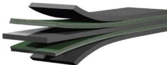
**Fig. 1 Typical Fiber Metal laminates [3]**
