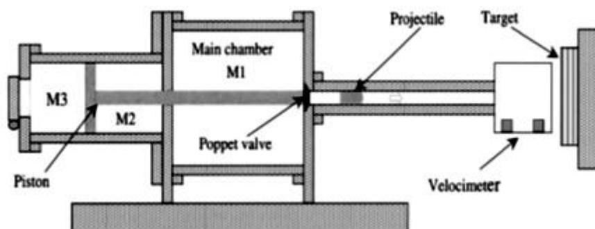
**Fig 7. Test arrangement for high Velocity Impact testing [21]**
