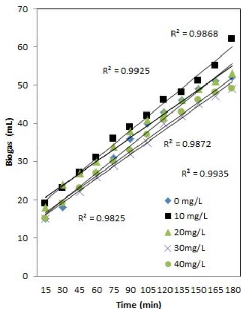
**Figure 1:** Evaluation of digestion performance in terms of cumulative biogas generation vs. time graph
