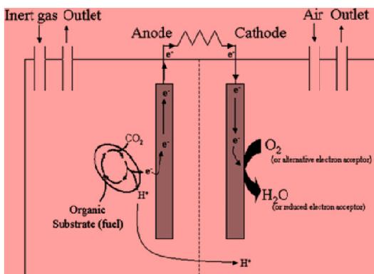
Fig. 1 Principle of a Microbial Fuel Cell.
